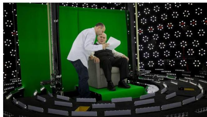
Figure 5 – Subject receiving direction in light stage used for generating 3-D imagery for holographic display
